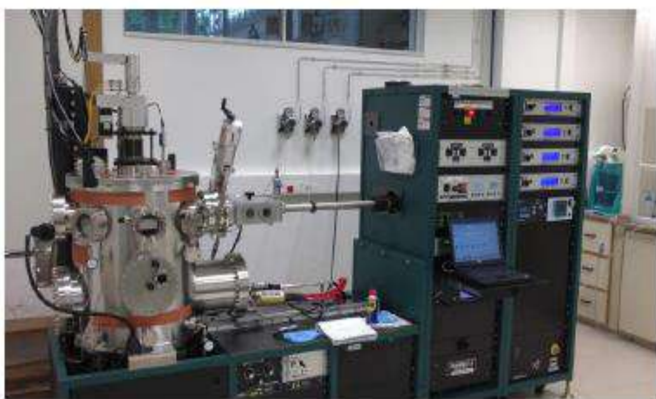
Fig. 1 –AJA international Inc. sputtering system
